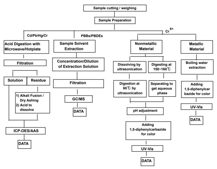
The samples were dissolved totally at the acid digestion step of the above flow chart for Cd,Pb,Hg Section Chief : Minkyu Park
