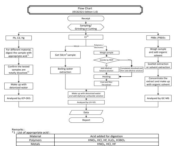
\*2 : The samples were dissolved totally by pre-conditioning method according to above flow chart.
