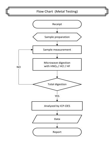
\*\* Remarks : The samples were dissolved totally by pre-conditioning method according to above flow chart.
